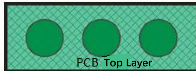
Fig. 6: Laying grid copper outside the top key sense element
