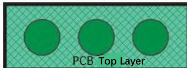
Fig. 5: Laying grid copper outside the top key sense element
